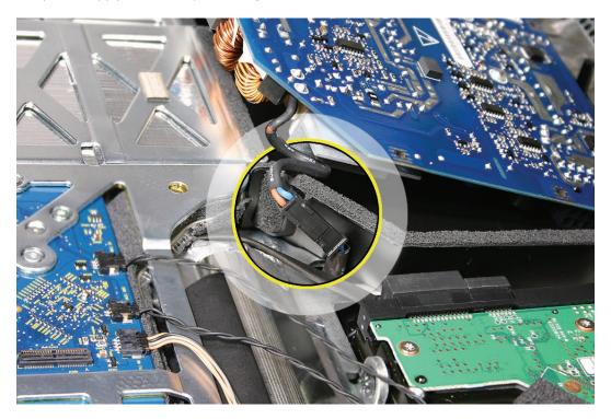
6. Lift the power supply from the rear housing.
